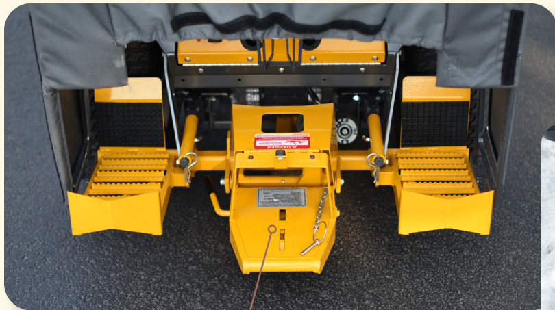
The Implement Hitch allows the Walker Mower to use implements
