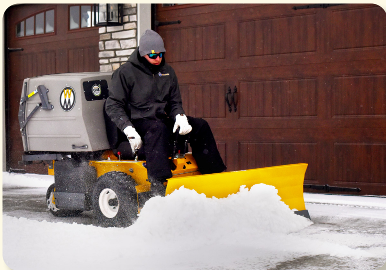
Replaceable steel wear edges
