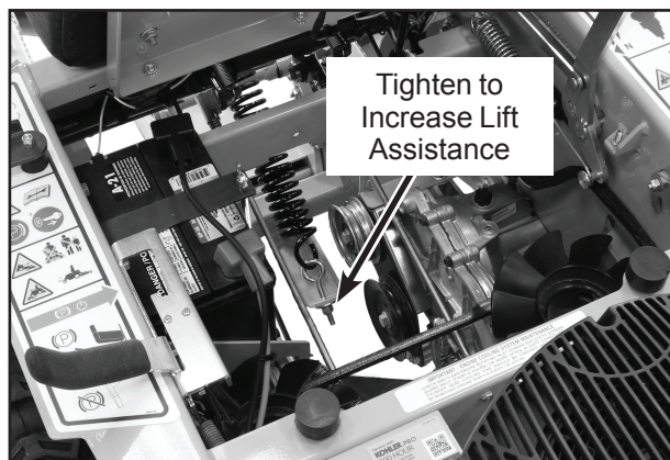
Lift Handle Assist Spring
