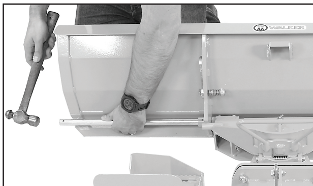
Feed Pivot Shaft Through Sockets
