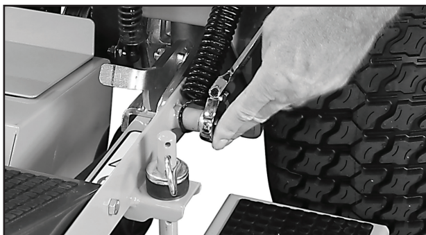
Remove Nut from Carrier Frame
